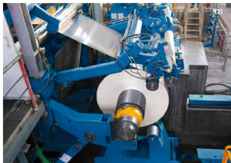
[1] | The first coil from the hot strip mill and [2] | winding the first coil in the cold rolling mill.
